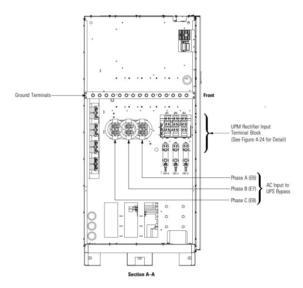
Figure 4-23. ISBM Section Power Terminal Detail AA – Separate Rectifier Feed
